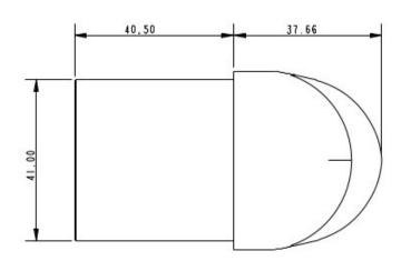
Details: The pivoting mast heel is designed for dinghies or small keelboats that have easily adjustable rigging whilst sailing. By allowing the mast heel to pivot it reduces loading points in the deck of the boat and spreads the forces more evenly. Having a pivoting mast heel also allows for a consistent mast bend profile resulting in more accurate rig setup. The A9151 is designed for use with the Paragon carbon mast. Made from Acetal.
