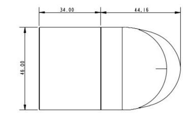
Details: The pivoting mast heel is designed for dinghies or small keelboats that have easily adjustable rigging whilst sailing. By allowing the mast heel to pivot it reduces loading points in the deck of the boat and spreads the forces more evenly. Having a pivoting mast heel also allows for a consistent mast bend profile resulting in more accurate rig setup. The A9152 is designed for use with the Super Spars carbon mast. Made from Acetal.
