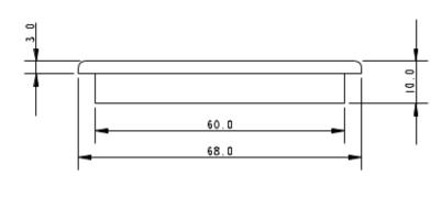
Details: CNC machined in-house. The A8040-56 has rope friendly radiused edges and a modern look. Perfect for bonding into a deck to allow a tidy pass through for control lines. Anodised dark grey.
