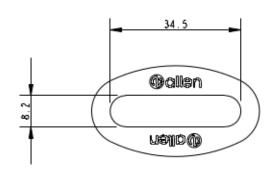
Details: CNC machined in-house. The A8040-34 has rope friendly radiused edges and a modern look. Perfect for bonding into a deck to allow a tidy pass through for control lines. Anodised dark grey.
