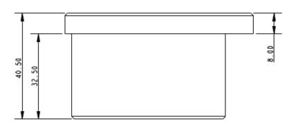
Details: The A9153 is designed for use with the Cumulus mast profile. The A9153 must also be paired with the A9150 & A9100. The pivoting mast heel is designed for dinghies or small keelboats that have easily adjustable rigging whilst sailing. By allowing the mast heel to pivot it reduces loading points in the deck of the boat and spreads the forces more evenly. Having a pivoting mast heel also allows for a consistent mast bend profile resulting in more accurate rig setup. Made from acetal.
