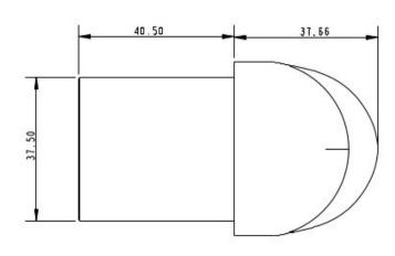
Details: The pivoting mast heel is designed for dinghies or small keelboats that have easily adjustable rigging whilst sailing. By allowing the mast heel to pivot it reduces loading points in the deck of the boat and spreads the forces more evenly. Having a pivoting mast heel also allows for a consistent mast bend profile resulting in more accurate rig setup. The A9150 is designed for use with the Selden carbon mast. Made from Acetal.
